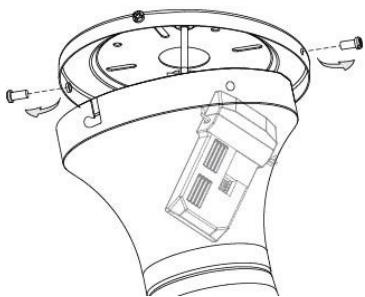
**5-1.** After the splicing has been made, gently place the receiver into the canopy and secure it in place using double-sided adhesive tapes which pre-adhered on the back of the receiver.
