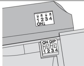
**3.** There is a frequency-setter in both the transmitter and receiver. This "DIP Switch" is a 4-key unit. All keys were set to "ON" position initially. Set the keys to a different code. Make sure the same numbered keys are switched to "ON" for both DIP Switches. Please note that the "ON" position may have a different orientation in each device.
