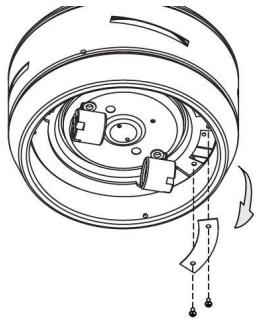
7. Remove the plate at light kit housing that covers the fan-shaped hole.
