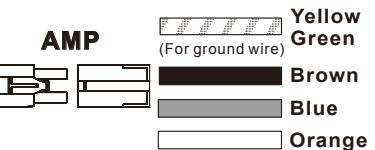
**4.** Make wire connections. Follow diagram above and make sure that all exposed wires are tightened by the screws on the terminal block.
