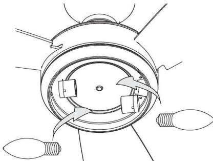
10. Install two proper lamps to the sockets (E27, B Type, max. 40W, not included).
