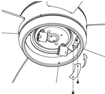
9. Re-attach the plate in place after blade installation is completed.
