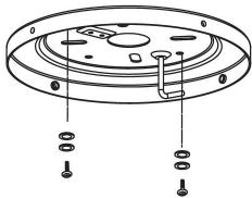
**1.** Pass the supply wires through the hole in the mounting bracket. Secure the mounting bracket to a ceiling joist or other structural ceiling element with two screws, spring washers and flat washers. Ensure that the support for the mounting bracket is capable of safely holding the moving weight of the fan.
