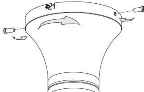
**6-1.** Push up the canopy until the two screws on mounting bracket are engaged with L type slot holes on canopy.
