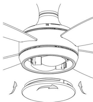
11. Install the glass shade onto the fan light housing by carefully rotating the lampshade clockwise.
